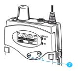
During FOCUS operation, the △/▼ rocker button ⑦ serves to adjust the relative levels of the two separate channels in the mixed mono signal (see "Stereo/FOCUS selection – ST-FOC" on page 27).
